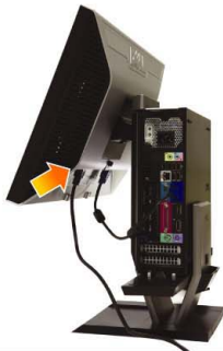
5 Connect the power cable firmly to the monitor as shown
